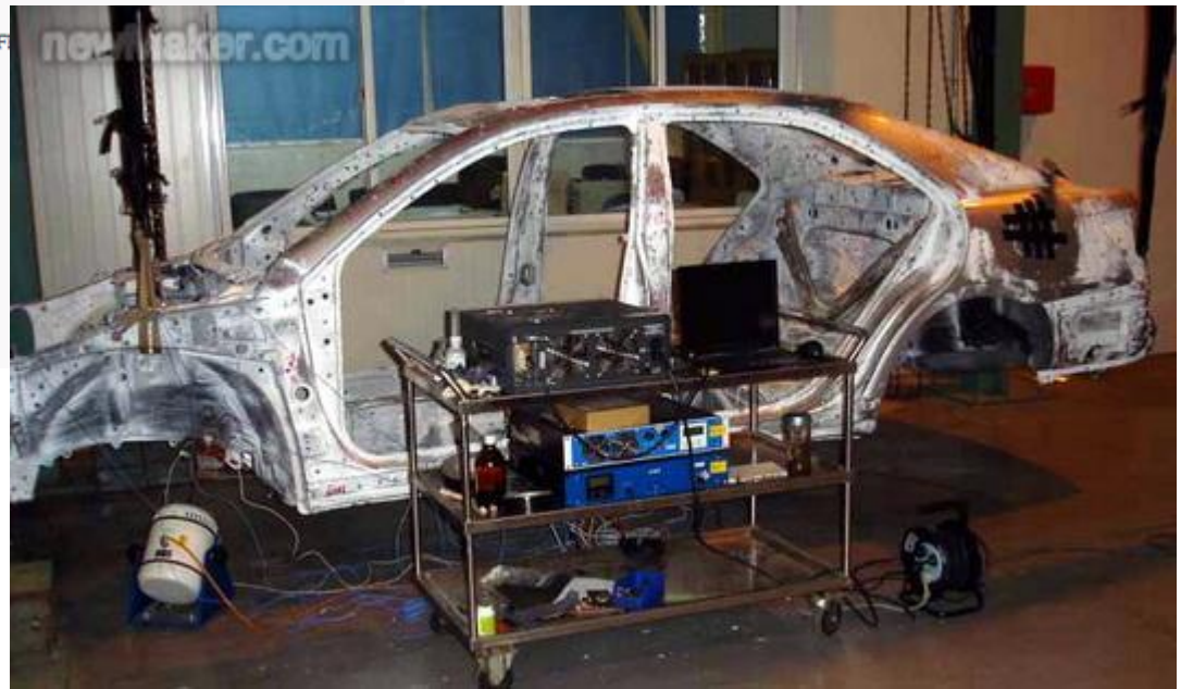
MAC4: FEA 41.3Hz, EMA 40.1Hz, Y向弯曲、前端扭转
